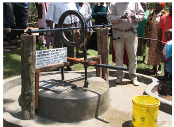
Newly refurbished well with rope and washer pump
